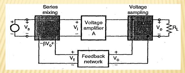
A transistor amplifier which uses the voltage series feedback is the common collector or emitter follower amplifier:
